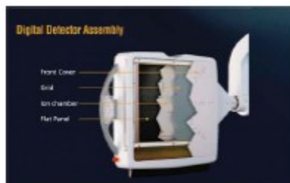
The UArm DR system utilizes a Varian 17" x 17" digital detector.
